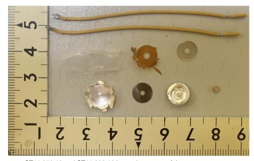
ST11 250 10 and ST11 200 10 internal structure of the motor protectors
