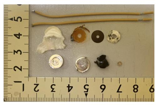
ST11 200 05 and ST11 060 05 internal structure of the motor protectors
